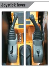
Simultaneous Control of Travel & attachment
