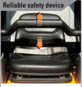
The adoption of a double safety gear minimizes the occurrence of accidents. A safety lever is to stop all functions when the operator departs from the unit ; the hydraulic line is to be cut off when the key is removed. The parking brake is to be
